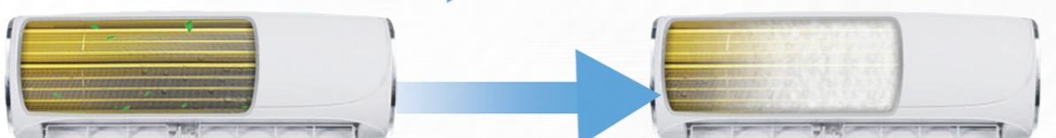
3.Evaporation removes residual moisture- from the evaporator
